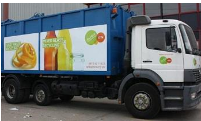
Figure 15: Split-bodied RCV for co-collection of food waste and glass (Sita)
